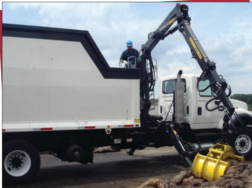
The new Kesla knuckleboom loader eliminates the physical demands of being a dead stock hauler.
