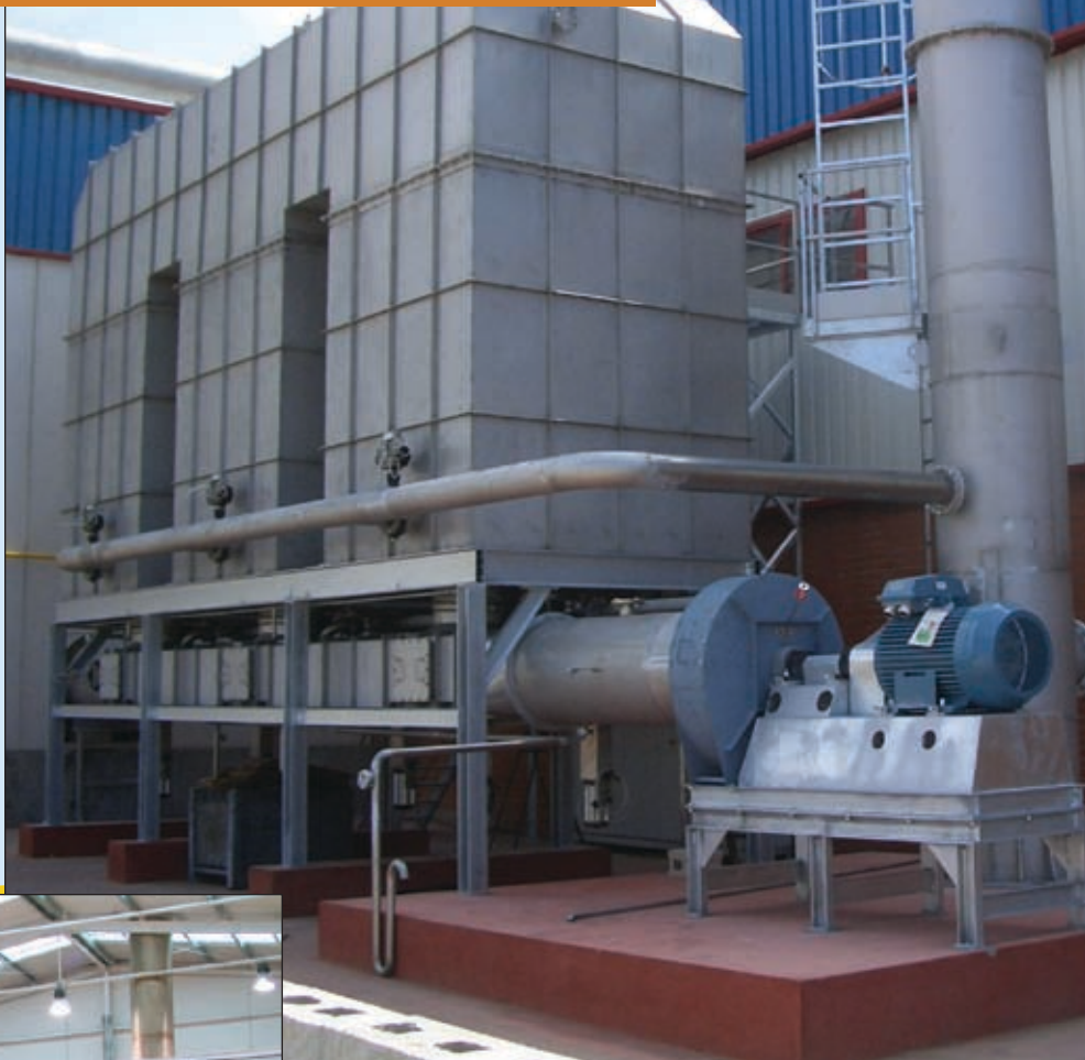
Top, a regenerative thermal oxidizer at a rendering plant.
