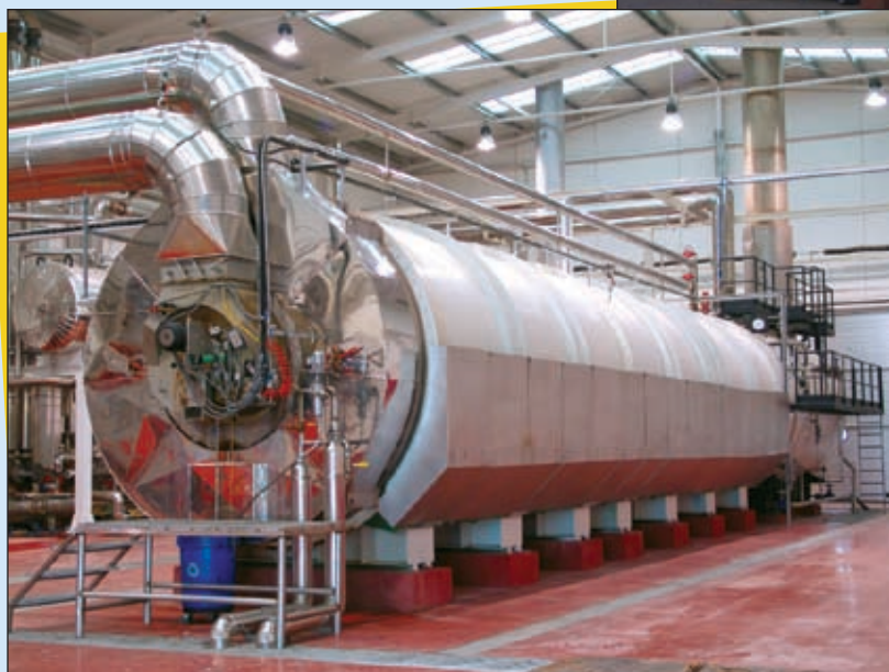
Top, a regenerative thermal oxidizer at a rendering plant.
