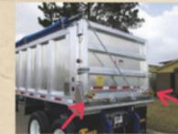
Ball valve drains, in gate or underbody
