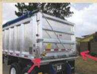
Ball valve drains, in gate or underbody
